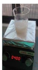
Figure 2.2 Preparation of ZnO seed solution
